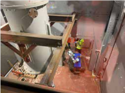
The CRADLE cell (shown above and left), located in the Amentum's laboratories in Birchwood Park, Warrington, is a mock-up of a nuclear fuel reprocessing cell for robotic decommissioning demonstrations. It features adjustable lighting, CCTV, network connectivity, industrial furniture, and a central 1-ton vessel, along with various pipes and beams. The cell is enclosed, with an adjacent elevated control room and observation window. Besides testing and demonstrations, it will support long-term experiments in a safe, realistic environment and be mirrored by a digital twin to explore integrated virtual and physical testing.
